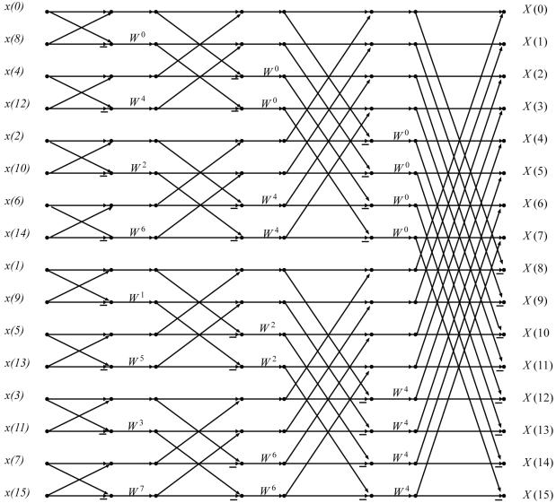
The benefit of using FFT over DFT is we need to compute only nlogn calculations as compared to n square calculations. The N Log N savings comes from the fact that there are two multiplies per Butterfly.
