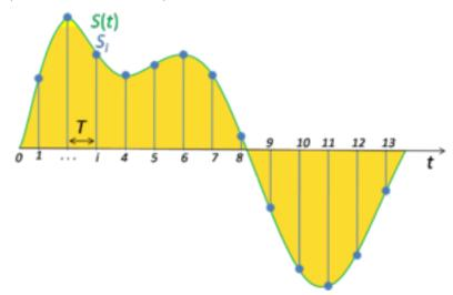
The sampling frequency or sampling rate, fs, is defined as the number of samples obtained in one second (samples per second), thus fs = 1/T. In practice, the continuous signal is sampled using an analog-to-digital converter (ADC).
