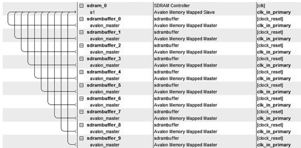
Figure 8-10: Multiple SDRAM buffer components in SOPC Builder
