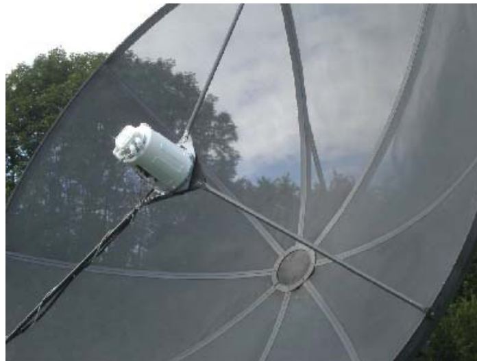
Figure 1 A 3m diameter dish with a 1420MHz feed
