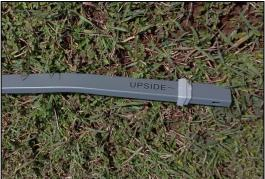
**Note:** Once the LNB Arm is in place do not try to remove it. The arm locks into place with the help of plastic locks. These can easily get damaged if the arm is pulled out after locking.
