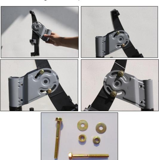
**Step 2:** Attach the dish holder to the dish using screws as shown. All the four nuts of the dish holder should be aligned properly with the fitting holes on the dish. After aligning the holder, simply screw in the appropriate screws (shown below) until they are sufficiently tight to hold the dish firmly.
